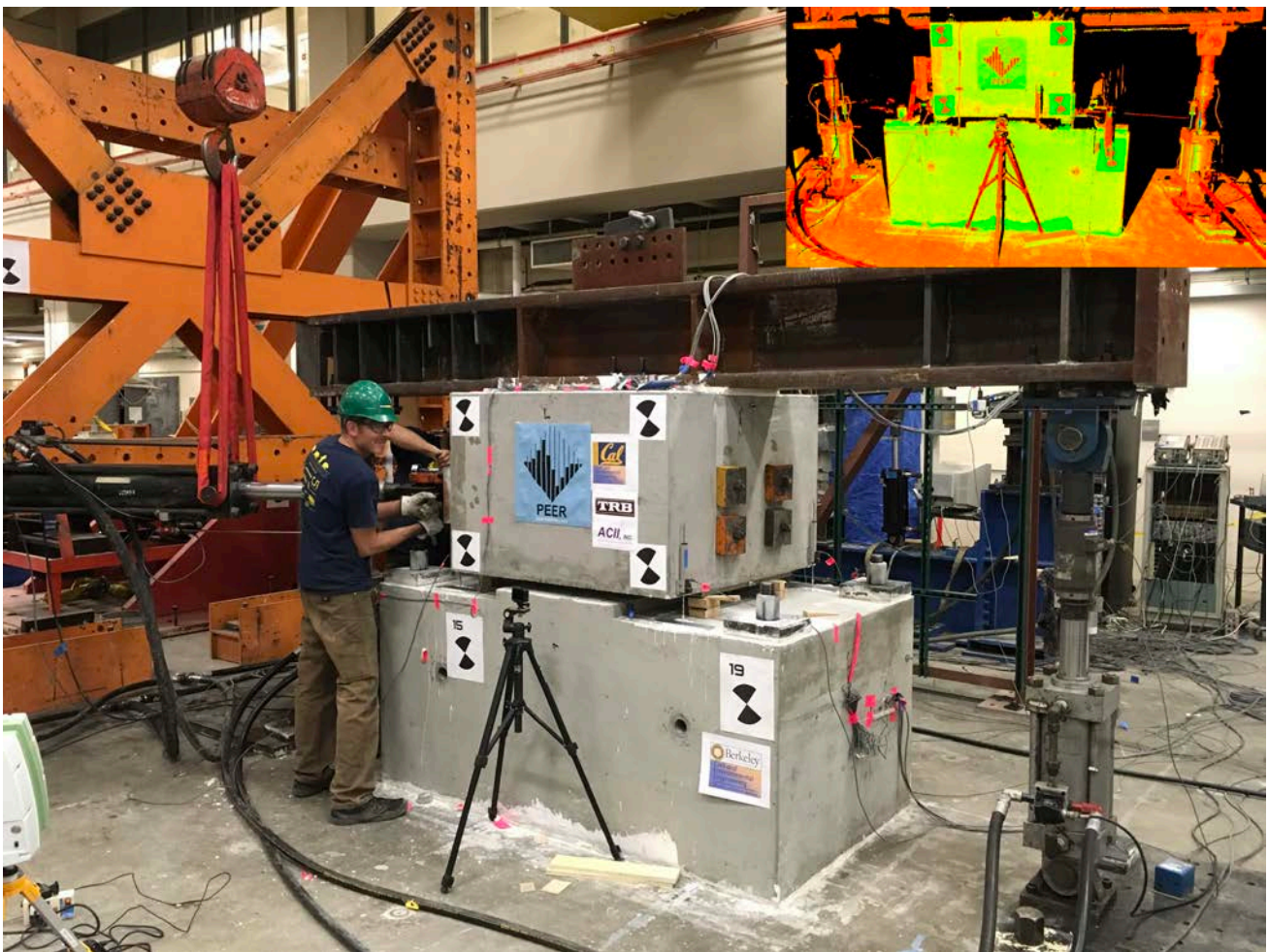
Fig. 26. Specimen assembly with two concrete blocks connected by V-connector of the VC1 group at the PEER Center test facility. The photo on the top right corner is a view by Terrestrial Laser Scanner that provides the displacement field of the entire system [13].
