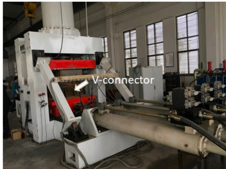
Fig. 28. The compression-shear test machine at the Fengzhe Laboratory, which is able to produce 10000kN (2248kips) compressive force along vertical and horizontal directions simultaneously.
