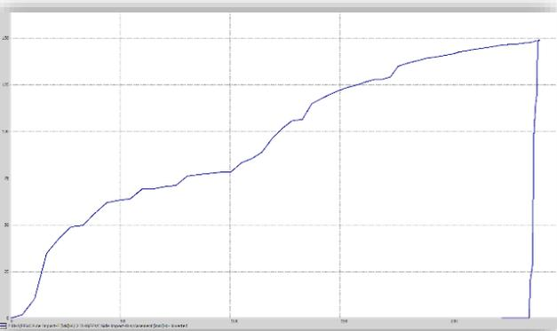
Barrier Force X [kN] vs Displacement Barrier X [mm]
