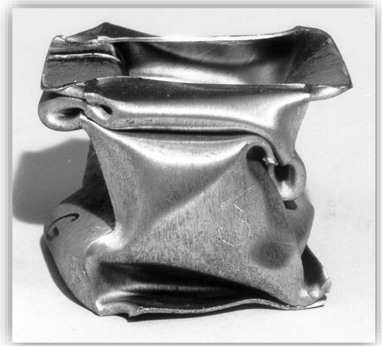
Irregular folding mode of column with wide side faces (large width, C , to thickness, t , ratio C/t ).
