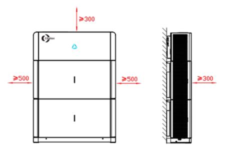
Figure 3-3 Installation space (unit: mm)
