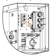
Figure 3-56 Insert the communication port
