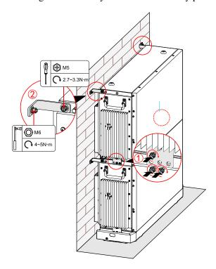
Figure 3-20 Tighten the top battery pack
