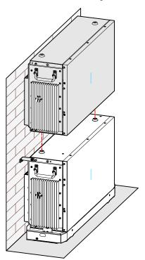
Figure 3-19 Place the battery pack
