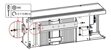
Figure 3-25 Tighten the inverter
