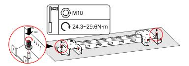
Figure 3-8 Fix the base module
