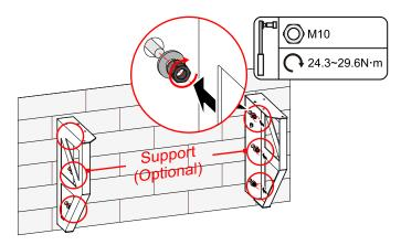
Figure 3-15 Mark the installation holes
