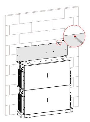
Figure 3-22 Mark the inverter drilling position
