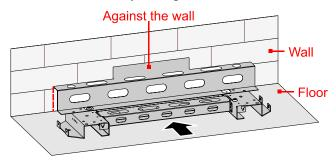
Figure 3-6 Auxiliary tool against the wall
