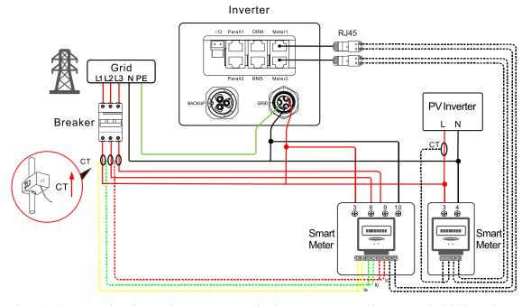
Figure 3-53 Connection diagram between communication smart meter and inverter and grid (three-phase + single phase)
