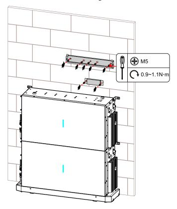
Figure 3-24 Install inverter wall bracket
