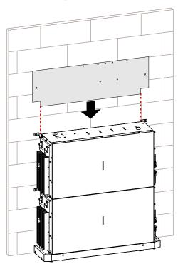
Figure 3-21 Place inverter positioning board
