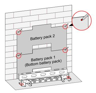
Figure 3-8 Mark the installation holes
