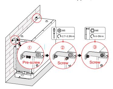
Figure 3-18 Fix the wall bracket a
