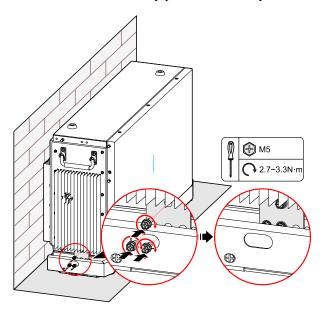
Figure 3-17 Fix the bottom battery pack with base
