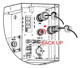
Figure 3-45 Insert the BACKUP terminal
