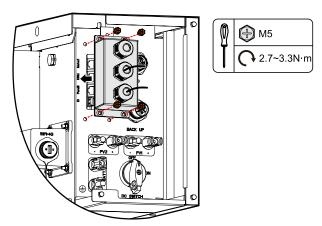
Figure 3-57 Screw the COM wiring cover
