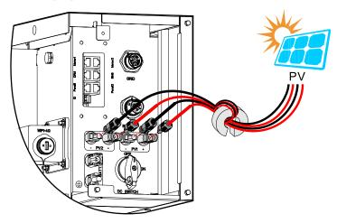
Figure 3-35 Connect the PV connector
