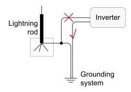
Figure 3-30 Grounding diagram of inverter
