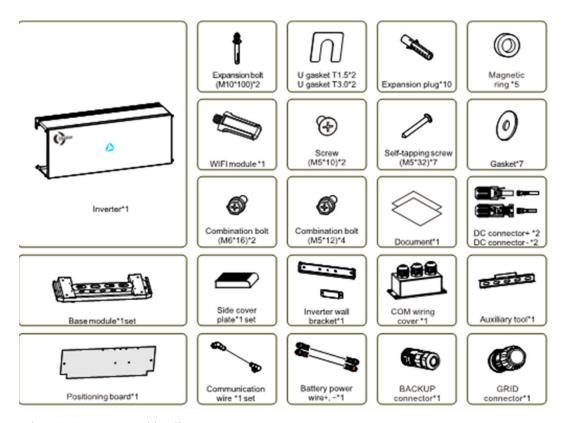
Figure 3-4 Inverter packing list
