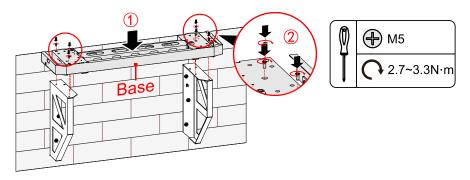
Figure 3-16 Assemble the support and base
