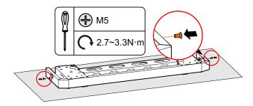
Figure 3-11 Fasten the cover plate
