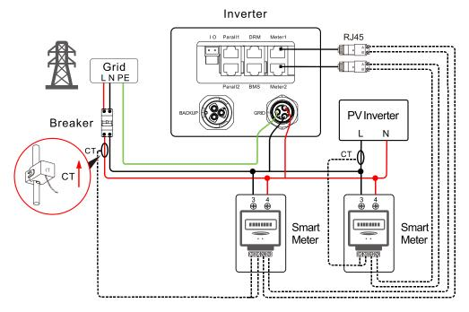
Figure 3-51 Connection diagram between communication smart meter and inverter and grid (single phase + single phase)
