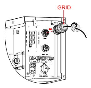
Figure 3-40 Insert the GRID terminal
