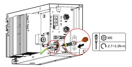
Figure 3-29 External grounding connection
