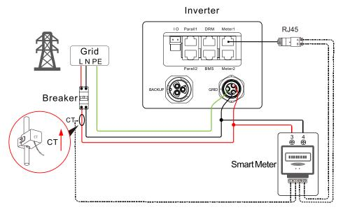
Figure 3-50 Connection diagram between communication smart meter and inverter and grid (single phase)
