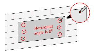
Figure 3-13 Mark the installation holes
