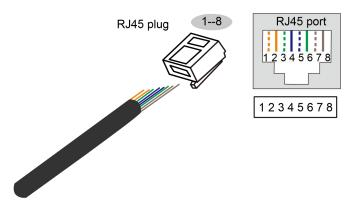
Pin definition of RJ45 plug: PIN 5: White blue - METER:B PIN 6: Green - METER:A
