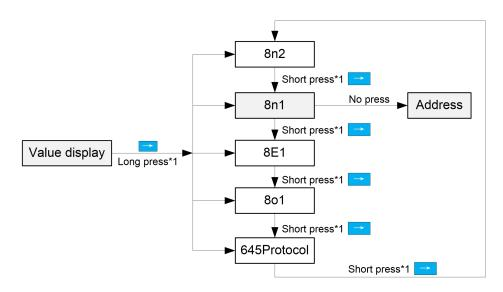
Figure 3-54 The setting of the smart meter address (single phase)
