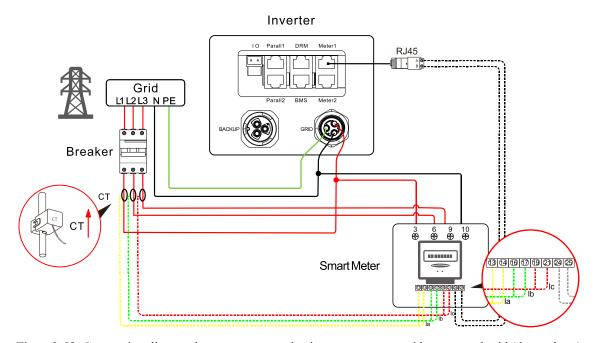
Figure 3-52 Connection diagram between communication smart meter and inverter and grid (three-phase)
