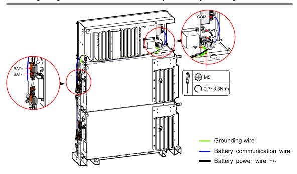
Figure 3-26 Battery pack external grounding wire connection
