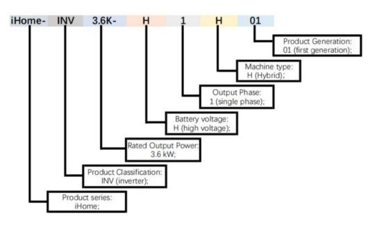
Figure 2-2 Model meaning of inverter
