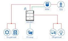
Figure2-5 Fully off-grid system
