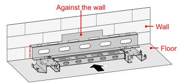
Figure3-6 Auxiliary tool against the wall
