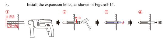
Figure 3-14 Install the expansion bolt (unit: mm)
