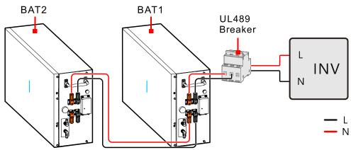
Figure3-23 Battery connection
