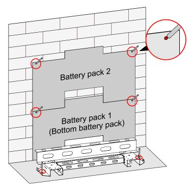
Figure 3-8 Mark the installation holes
