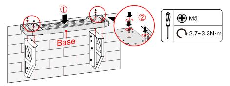
Figure 3-16 Assemble the support and base
