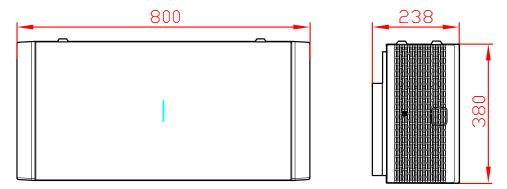
Figure2-4 Battery size (Unit: mm)
