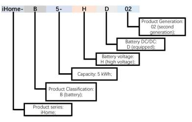
Figure 2-2 Model meaning of battery
