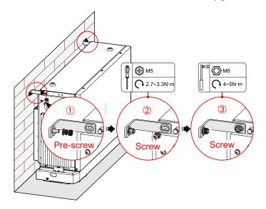
Figure3-18 Fix the wall bracket a
