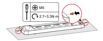
Figure 3-11 Fasten the cover plate
