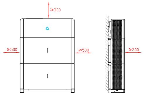
Figure3-3 Installation space (unit: mm)
