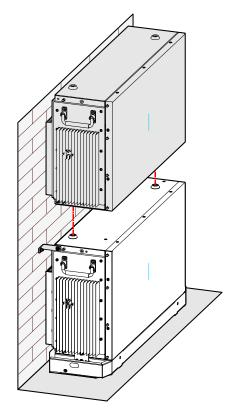
Figure 3-19 Place the battery pack
