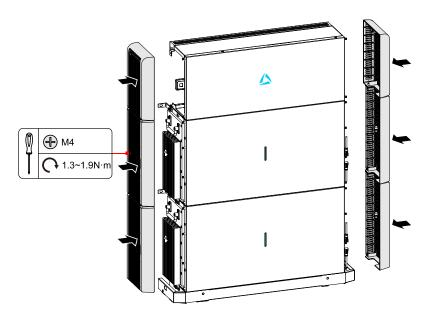
Figure 3-24 Tighten the wiring cover plate
