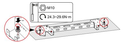
Figure 3-8 Fix the base module
