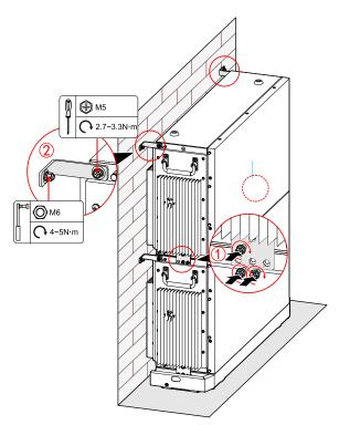
Figure 3-20 Tighten the top battery pack
