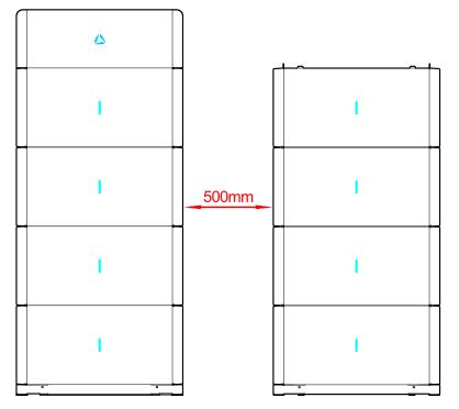
Figure 3-21 Distance between the batteries
