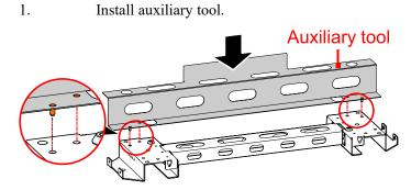
Figure3-5 Install auxiliary tool
