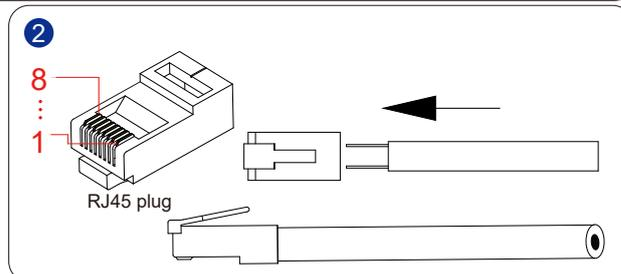
3. Crimp the RJ45 plug with a wire crimper.
