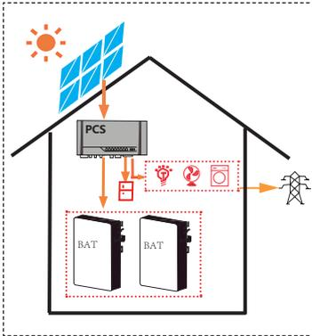
The energy produced by PV is optimized to supply loads. The excess energy is used to charge battery, then export to grid.
