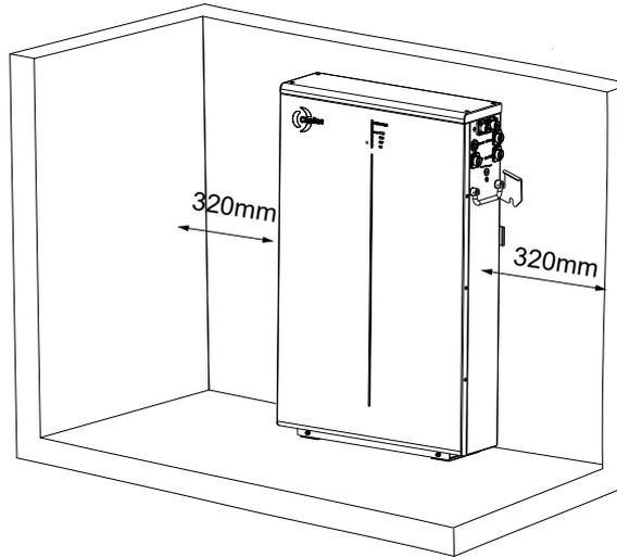
3. Use pencil to mark where the notches of two latches are and confirm the two drilling spots. Move battery away.
