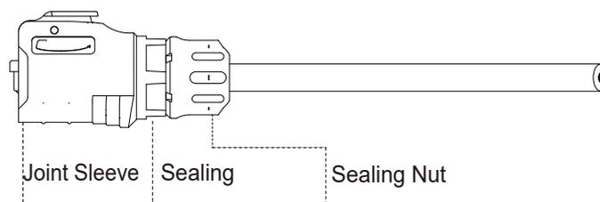
1. Strip cable sheaths for  $15 \pm 0.5$ mm first and insert sealing and sealing nut along the cable.
