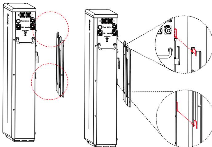
3. Rotate the left latch rightward until the notch locks limiting pin, and rotate the right latch leftward until the notch locks limiting pin too.
