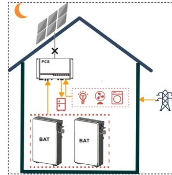
Battery powers loads at nighttime when there is no PV. If battery energy is insufficient, it can power loads together with grid.
