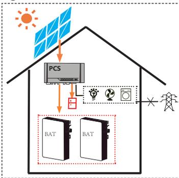
When grid falls, battery and PV can power loads.
