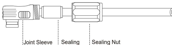
1. Strip cable sheaths for  $20 \pm 0.5$ mm and insert sealing and sealing nut along the cable.
