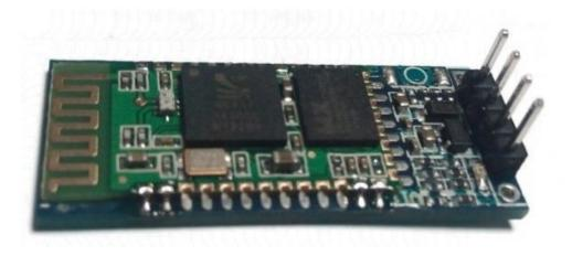
1,Core module uses HC-06, leads from the module interface includes VCC, GND, TXD, RXD, reserve LED status output pin, the microcontroller can be judged by the foot state Bluetooth has connected KEY pin slave invalid.
