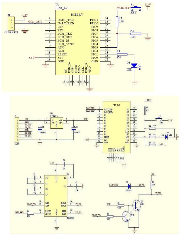
HC-06 master device has a function of remembering the last paired slave device. As a master device, it will search the last paired salve device until the connection is built. But if the WAKEUP bottom is pressed, HC-06 will lose the memory and research the new
