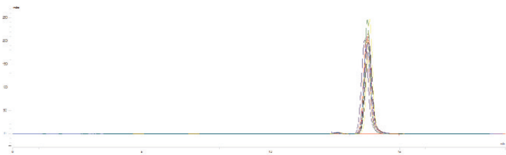
Column Efficiency after Repeated Packing Test of WePure XP Hybrid packing media
