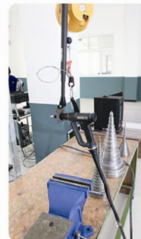
扭矩检测仪 To test the torque on basis of certain rotate speed
