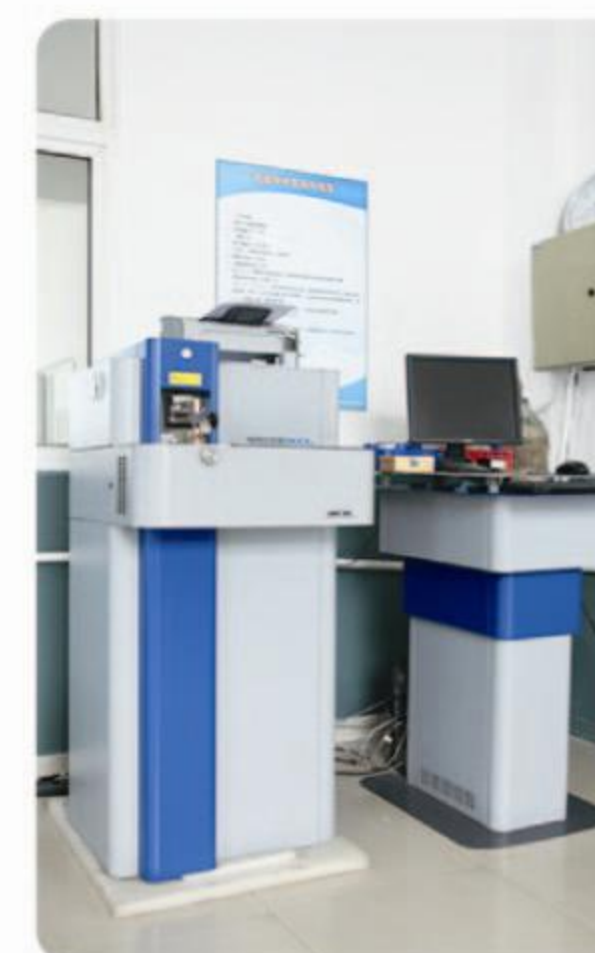
光谱仪 To test the composition of the raw material
