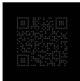
2D code reconstructed image with 0th order light suppression
