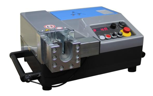
Cutting ring assembly and flaring machine
