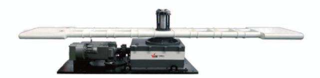
CMT series centrifugal constant acceleration tester is used to test articles under extreme acceleration conditions based on standard like MIL-STD-810F, MIL-STD-202 and IEC68-2-7. It is most suitable for testing electronic components or devices. Under high g effect on microcircuits, to check adaptability and reliability of wiring and the internal structures. It may expose mechanical and structural defects that are not found with vibration and shock tests.
