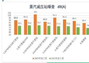
噪声结果显著降低。在J1509阀门20%开度时，所有测点噪声均在80 dB(A)以下。The noise results are significantly reduced. The noise at all measuring points is below 80 dB(A) when the J1509 valve is 20% open.
