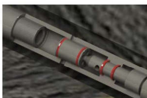
2、开泵 (旁通关) Pump started (bypass off)
