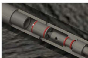
1、停泵 (旁通关) Pump stopped (bypass off)
